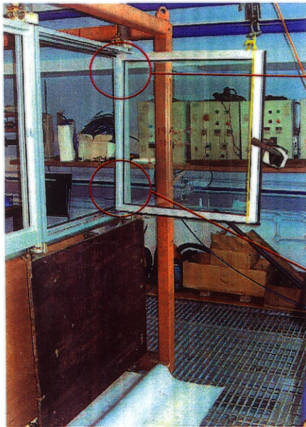
Photo 3: Window #2 with one pair of safety devices – initial test setup
